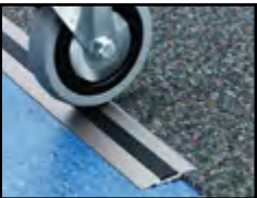
DT024 Sheet Vinyl Transition SAFETY TRANSITION FOR USE BETWEEN 2MM SHEET VINYL AND CARPET. PRE-DRILLED AND COUNTER-SUNK HOLES FOR #4 SCREW 82° INSERT WIDTH: 13MM FINISH: EA, EN, BRZ, EBLK
