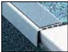
AA123 2" Right Angle Drop SAFETY STAIR WITH PRE-DRILLED AND COUNTER-SUNK HOLES FOR #4 SCREW 82° INSERT WIDTH: 53MM FINISH: EA, EN, BRZ, EBLK
