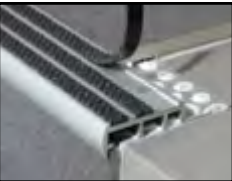
AA351 Ceramic Stair Nose SAFETY STAIR WITH PRE-DRILLED AND COUNTER-SUNK HOLES FOR #4 SCREW 82° INSERT WIDTH: 13MM X 3 FINISH: EA, EN, BRZ
