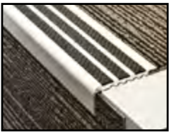
AA346 1 3/8" Right Angle Drop SAFETY STAIR WITH PRE-DRILLED AND COUNTER-SUNK HOLES FOR #4 SCREW 82° INSERT WIDTH: 13MM X 3 FINISH: EA, EN, BRZ
