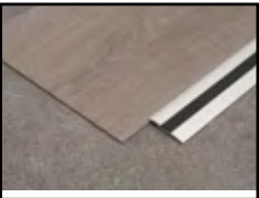
DT027 Carpet to LVT Transition SAFETY TRANSITION FOR USE BETWEEN 3MM LVT AND CARPET. PRE-DRILLED AND COUNTER-SUNK HOLES FOR #4 SCREW 82° INSERT WIDTH: 13MM FINISH: EA, EN, BRZ, EBLK
