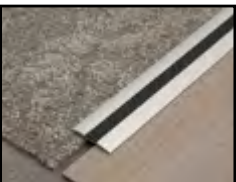
DT029 Carpet to LVT Transition SAFETY TRANSITION FOR USE BETWEEN 5MM LVT AND CARPET. PRE-DRILLED AND COUNTER-SUNK HOLES FOR #4 SCREW 82° INSERT WIDTH: 13MM FINISH: EA, EN, BRZ, EBLK
