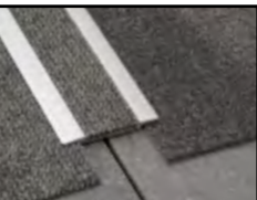
DT026 Safety Joiner SAFETY JOINER FOR USE WITH CARPET TILE. PRE-DRILLED AND COUNTER-SUNK HOLES FOR #4 SCREW 82° FINISH: EA, EN, BRZ, EBLK
