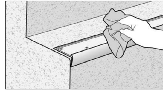
Ensure the aluminum channel is clean from dust, residues and debris. Wipe down with a cleaning solvent (Isopropyl Alcohol or similar).
