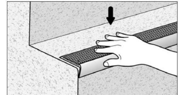
Install by placing the Insert into the nosing and pressing into place without undue stretching.
