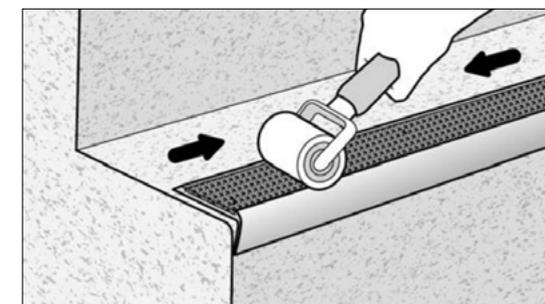
Once in place, roll over the Insert to ensure consistent adhesion and a secure bond. Please take care not to stretch the Insert when rolling. Installation is now complete.
