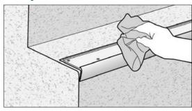
Ensure the aluminum channel is clean from dust, residues and debris. Wipe down with a cleaning solvent (Isopropyl Alcohol or similar).
