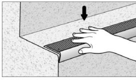
Install by placing the Insert into the nosing and pressing into place without undue stretching.
