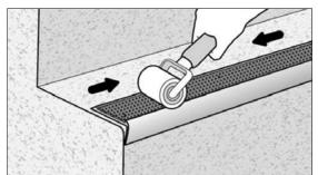
Once in place, roll over the Insert to ensure consistent adhesion and a secure bond.
