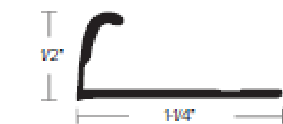
CM 201 1/2" PREMIUM PINLESS CLAMPDOWN FINISH: HMF, HB, HEA, HN, HBDB, CVG, HBRZ, HMF-FLEX, HB-FLEX, HEA-FLEX, HN-FLEX
