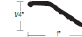
CM 313 1" STANDARD BINDER BAR FINISH: HMF, HB, HEA, HN, HBDB, CVG, HBRZ
