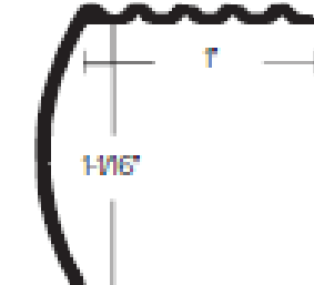
CM 611 1" STANDARD STAIR NOSING FINISH: HMF, HB, HEA, HN, HBDB, CVG, HBRZ
