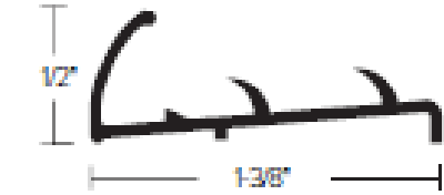
CM 3703 1/2" STANDARD PIN CLAMPDOWN FINISH: HMF, HB, HEA, HN, HMF-FLEX, HB-FLEX, HN-FLEX
