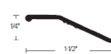
CM 312 1 - 1/2" STANDARD BINDER BAR FINISH: HMF, HB, HEA, HN, HBDB, CVG, HBRZ, OAK, CHERRY, GUNSTOCK
